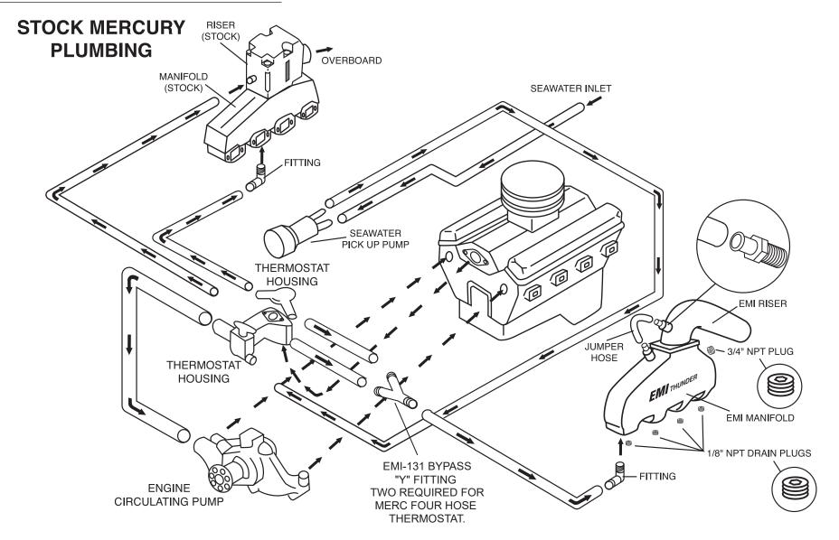
WATER MUST BE FLOWING THROUGH THE MANIFOLD AT ALL TIMES! CHECK THE MANIFOLDS UPON START UP TO INSURE THAT THEY STAY COOL. WATER MUST EXIT THE EXHAUST WITHIN 1-2 MINUTES AFTER STARTING THE ENGINE. FAILURE TO HAVE MAXIMUM WATER FLOW TO THE MANIFOLDS CAN CAUSE SEVERE INTERNAL DAMAGE AND WILL VOID THE WARRANTY! APPLY A THIN COAT OF HIGH TEMP SEALANT TO BOTH SIDES OF RISER GASKET.
