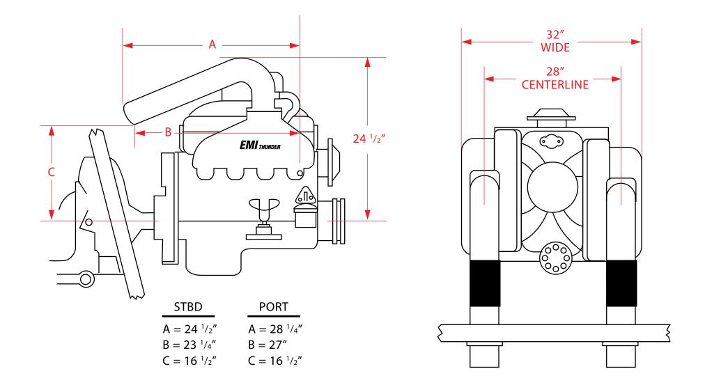
NOTE: These dimensions may vary slightly and should only be used as a guide for determining fitment of EMI Thunder exhaust to your boat.
