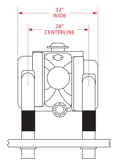
NOTE: These dimensions may vary slightly and should only be used as a guide for determining fitment of EMI Thunder exhaust to your boat.
