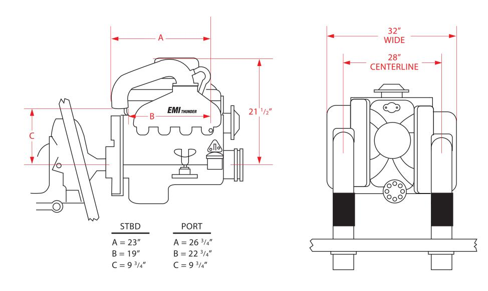
NOTE: These dimensions may vary slightly and should only be used as a guide for determining fitment of EMI Thunder exhaust to your boat.
