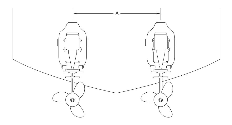
Provide dimension "A" when ordering a Tie Bar assembly.
