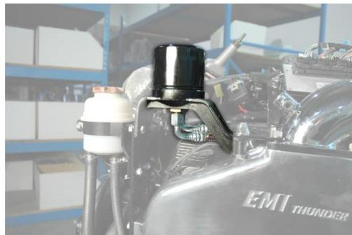
40. Tighten up the riser studs and nuts approx. **20 lb. of torque**
