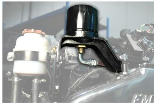
36. Bolt assembly to manifold, using bolts supplied, bolt bracket to lower front of manifold and upper front bolts on riser, do not tight yet.
